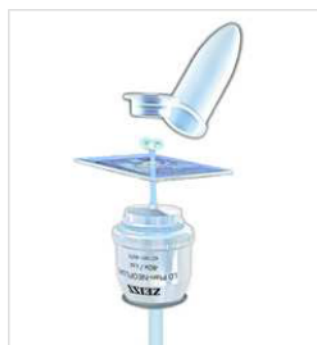
Figure 4 Principle of ZEISS non-contact laser microdissection technology: a laser isolates the desired sample and transfers it into a collection cap. Auto-documentation of sperm cells before LCM and after LCM, indicating the successful transfer to the collection cap.
