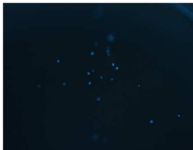
Figure 5 View with 5x objective in the collection cap. The PEN membrane exhibits strong autofluorescence when excited with light around 400nm (e.g. DAPI-Filter). This allows easy identification and verification of the isolated and captured sample in the cap. Here, 25 sperm cells have been successfully captured via LCM.
