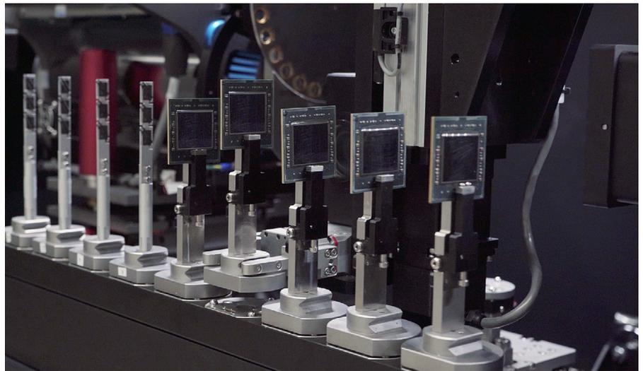
*ZEISS Autoloader option enables you to program up to 70 samples at a time to run sequentially.*
